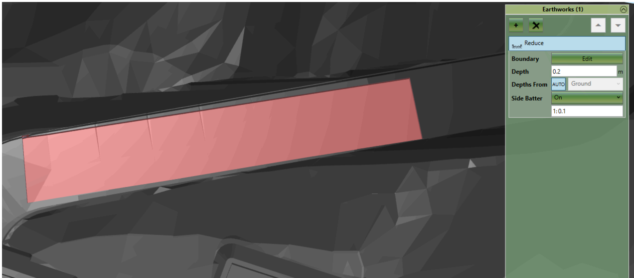
Defining a section of road, milled to a depth of 200mm with a Reduce Element.
